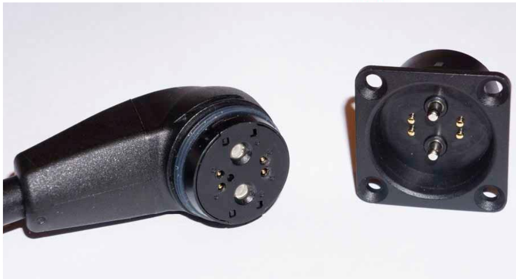
EnergyBus charge connector which was released by March 2012, which is based on the proven beta version which has been sold already about 0,5 Million times.
