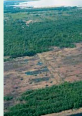
In the Barloh section the firm that had been removing the peat additionally closed the ring-shaped drainage trench as well as numerous slit trenches so that the water could once again be retained in the moor.
